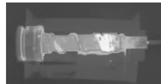
Temperature distribution using standard coiled cable heater.
