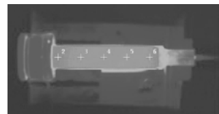
Temperature distribution using thick film heating technology.
