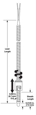
Adjustable armor thermocouple fits a large range of hole depths. Bends to any angle, eliminating the requirement to stock numerous styles. Stainless steel hose offers additional lead protection in demanding applications.
