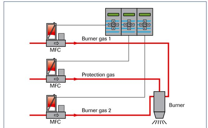
Burner control using Mass Flow Controllers brings many advantages compared to conventional systems, where flow is adjusted through needle valves. When burner orifices get clogged or when gas supply pressure varies, an MFC will automatically adapt to the changed conditions. For the control of relatively large flows with low differential pressure, which is typical for natural gas or CH<sub>4</sub>, Bronkhorst High-Tech offers mass flow meters with separate pressure compensated bellows valves.
