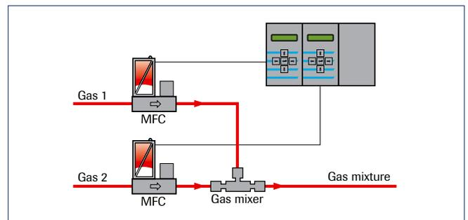
MFC's are often used to make precise and stable mixtures of two or more gases. A Bronkhorst PS/Readout system can be applied to maintain the ratio of mixed gases by operating in master-slave mode. In the example above, the flow range of gas 1 is much smaller than the other. For this purpose Bronkhorst High-Tech developed a gas mixer, to guarantee a homogeneous gas mixture.
