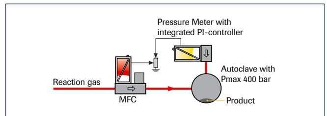
Flow control is often combined with the control of reactor pressure, using an EL-PRESS back pressure controller, or as depicted, an EL-PRESS Pressure Meter with integrated PI-controller. Typical applications: high pressure hydrogenation systems and autoclave processes using a 400 bar rated Mass Flow Controller with Vary-P control valve.
